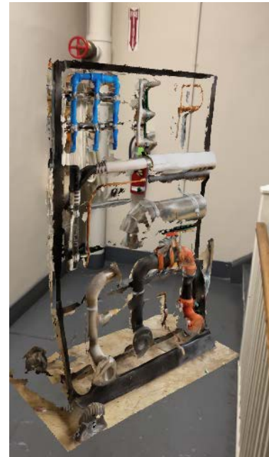
iPhone Pro AR relocation to check clearance needed to get skid up stairs
